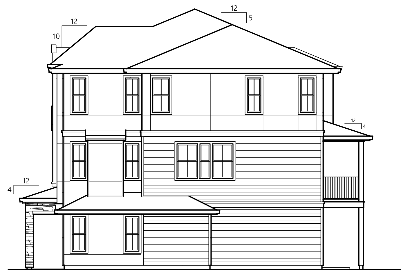
Building 1 (Lots 156-158) 1/8" = 1'-0" ENHANCED SIDE ELEVATION CONTEMPORARY FRENCH
