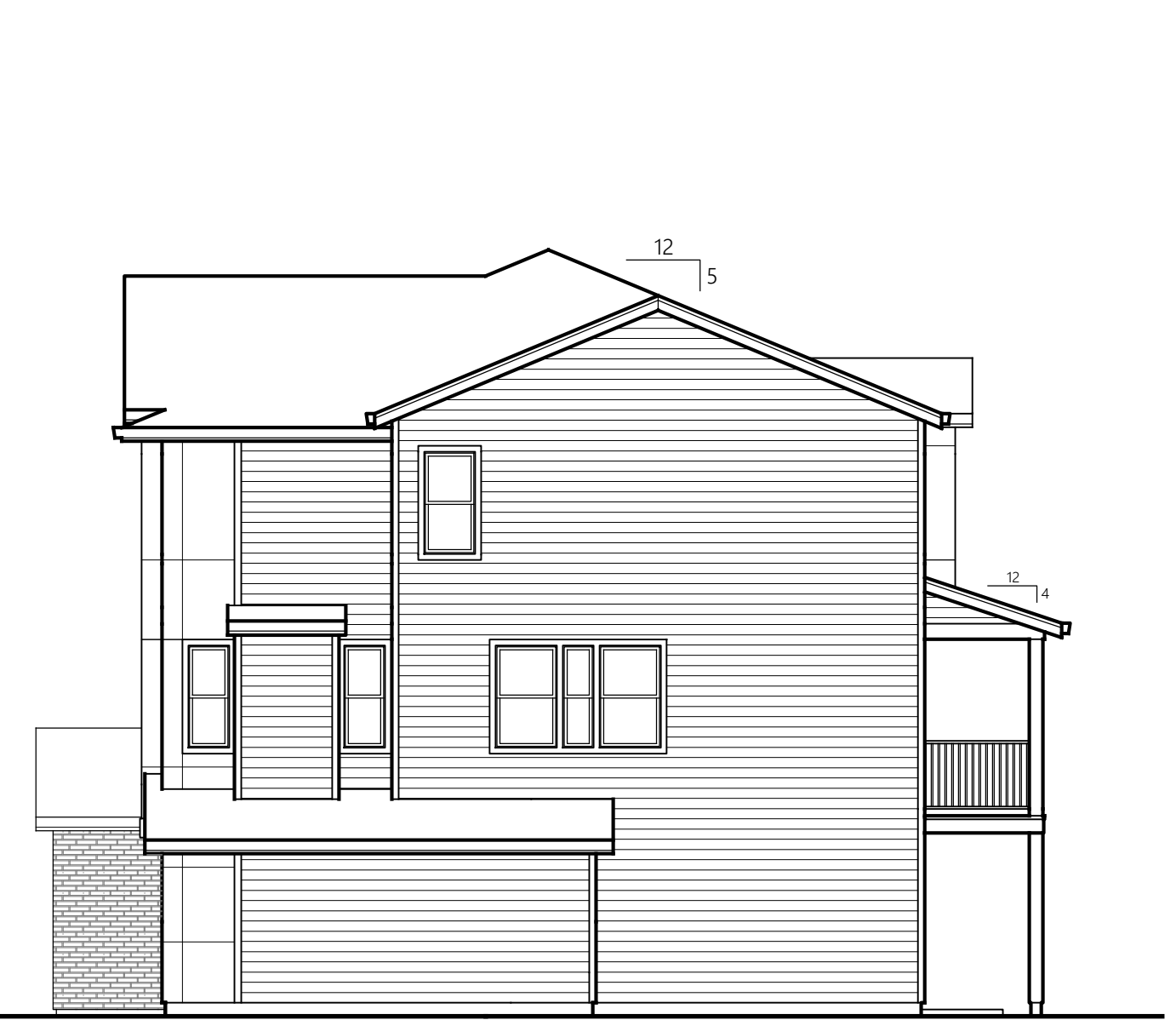
Building 3 (Lots 164-168) 1/8" = 1'-0" SIDE ELEVATION CONTEMPORARY TUDOR
